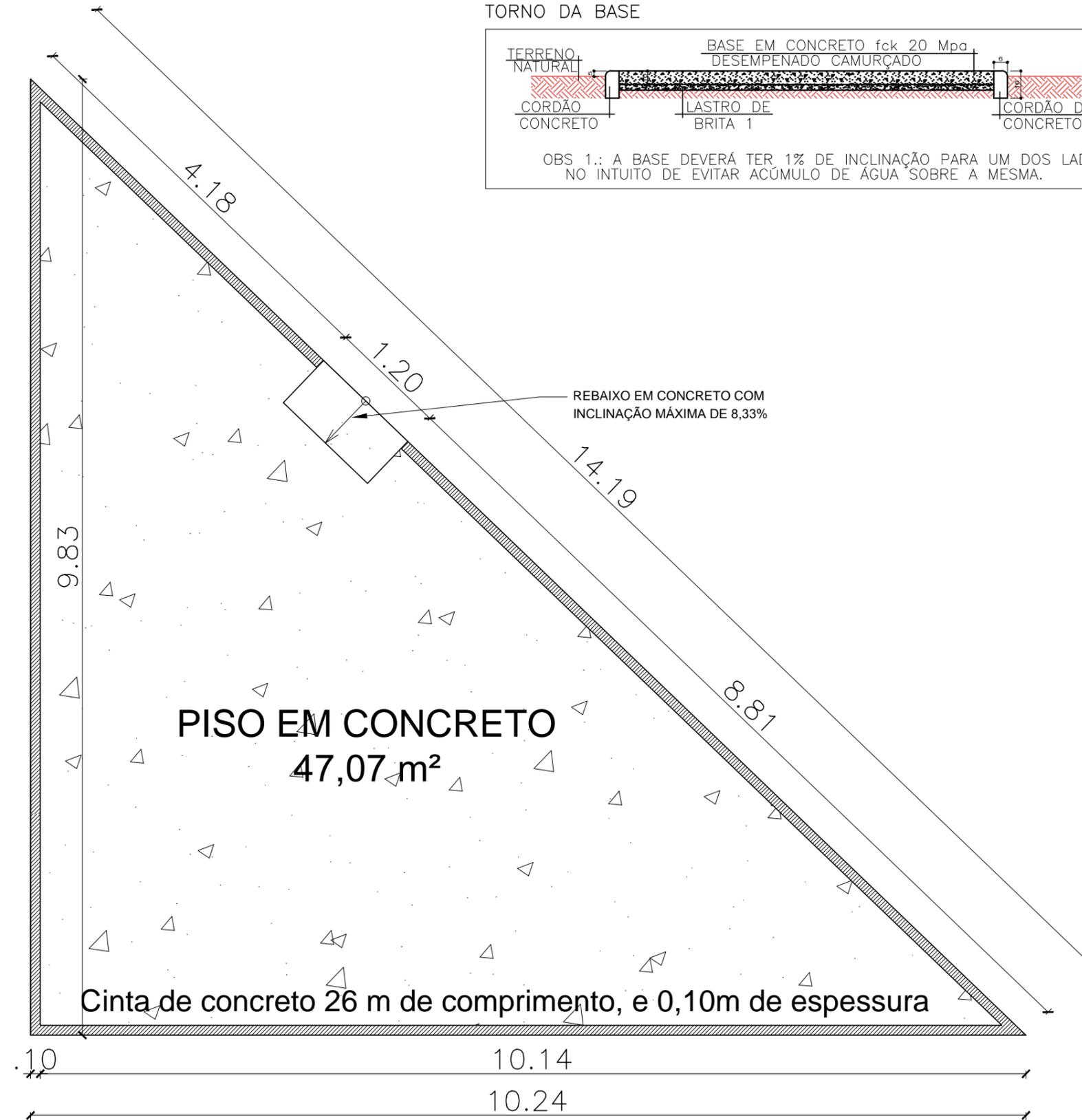
PLANTA BAIXA - PISO EM CONCRETO A CONSTRUIR SEM ESCALA
